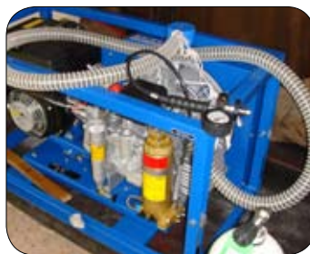
Photo 19: Typical HP compressor.
