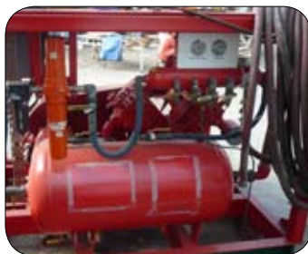
Photo 18: Typical LP air compressor.
