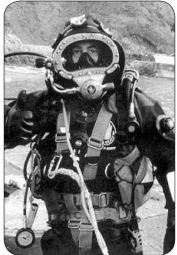
Photo 22: Demonstrating the use of SCUBA with lifeline and communications line.
