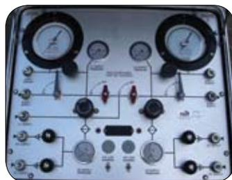
Photo 5 : Typical portable air supply panel.
