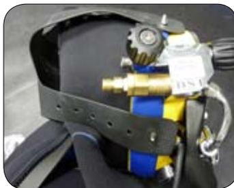
KMB 18 Band mask coupled with side block assembly
