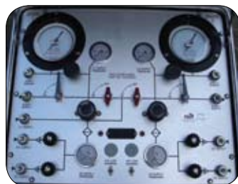
Photo 5 : Typical portable air supply panel.
