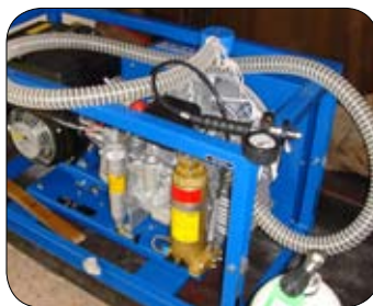
Photo 19: Typical HP compressor.
