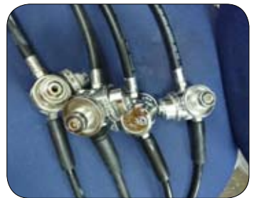
Photo 15 : Divers bail out bottle first stage regulators.
