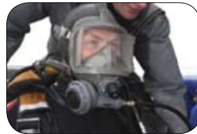
Full face mask; no side block assembly
