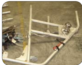
Diver recovery davit
