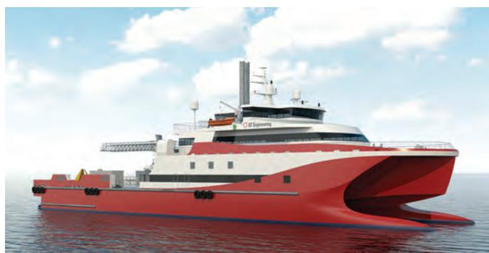
ST Engineering Marine's dual fuel LNG catamaran fast crew boat is designed for offshore operations.
